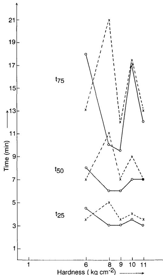
Fig. 1. Plot of compression hardness vs time to release of 25% ( $t_{25}$ ), 50% ( $t_{50}$ ) and 75% ( $t_{75}$ ) of piroxicam. Polymorph  $\alpha$  O, polymorph  $\beta$  x.
