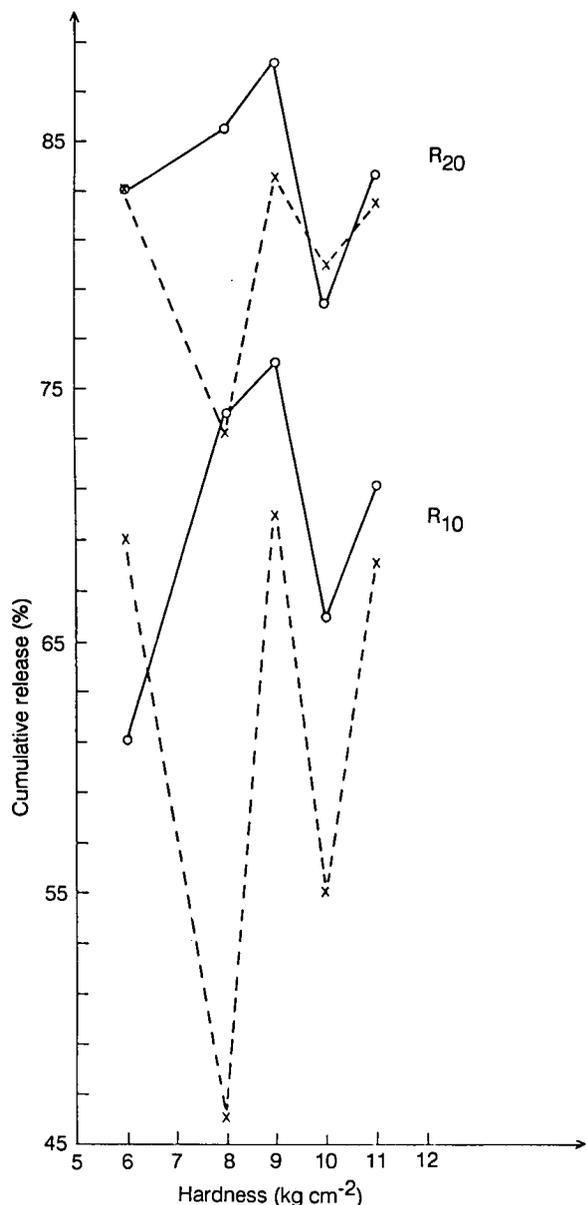
FIG. 2. Plot of compression hardness vs release of piroxicam in the first 10 ( $R_{10}$ ) and 20 ( $R_{20}$ ) min. Polymorph  $\alpha$   $\circ$ , polymorph  $\beta$   $\times$ .
