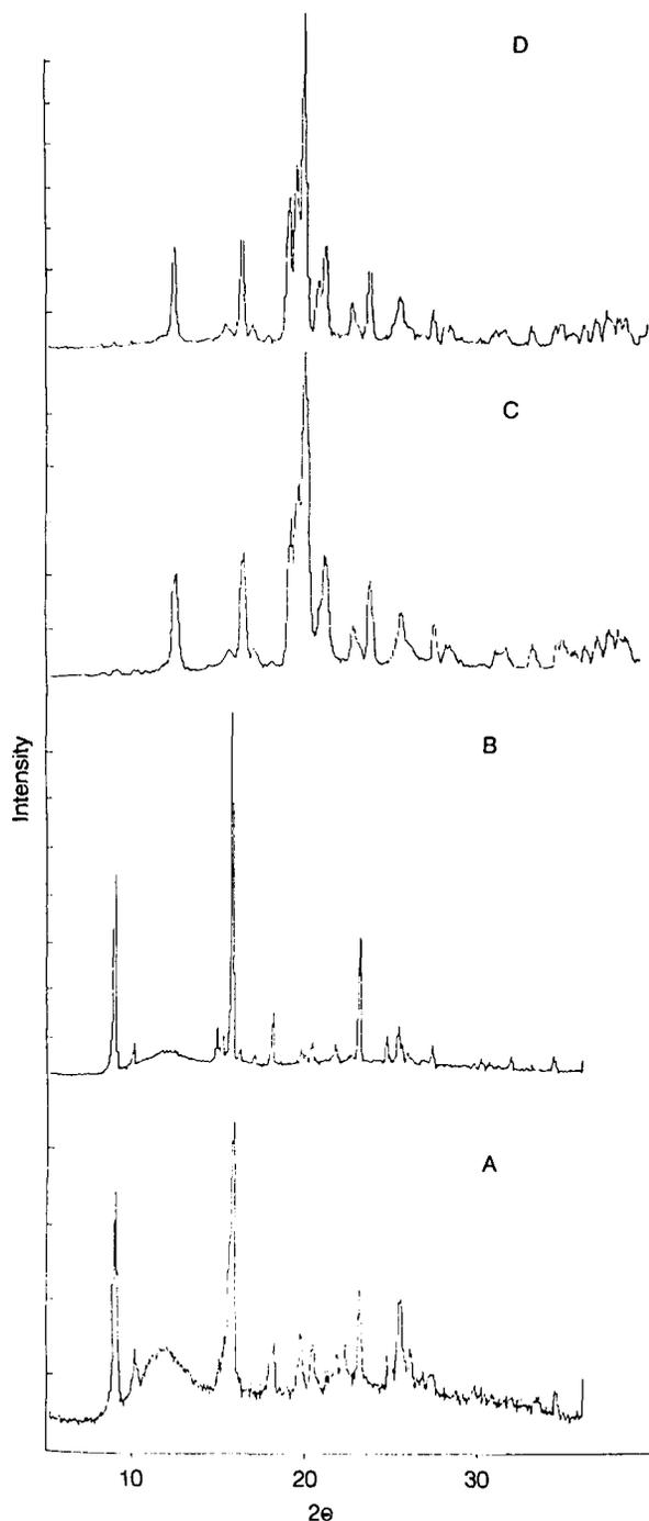
FIG. 4. Powder X-ray diffractograms of A, polymorph  $\alpha$ , B, polymorph  $\beta$ , C, LT $\alpha$ 9, and D, LT $\beta$ 9.
