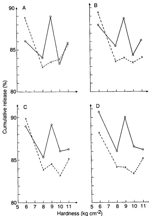
FIG. 3. Plot of compression hardness vs release of piroxicam in (A) 30 min ( $R_{30}$ ), (B) 40 min ( $R_{40}$ ), (C) 50 min ( $R_{50}$ ) and (D) 60 min ( $R_{60}$ ). Polymorph  $\alpha$   $\circ$ , polymorph  $\beta$   $\times$ .
